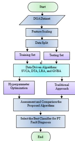
Fig. 2. Flowchart of the Data-Driven Algorithms Process
