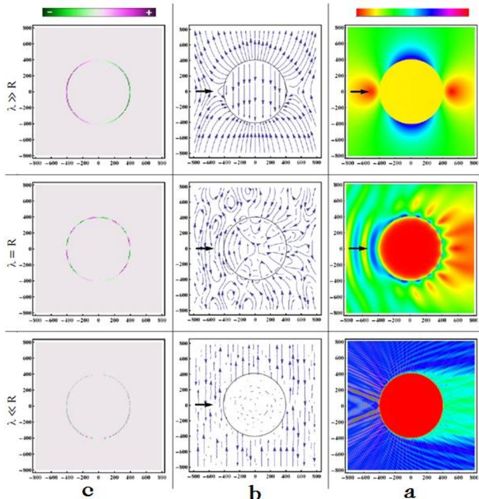
Fig. 4. Distribution of the field in and around, a plasmonic nanowires for  $\lambda \gg R$ ,  $\lambda = R$  and  $\lambda \ll R$ . The electric field, (a) field lines, (b) and distribution of the charge density, (c). (axes are in nanometer).
