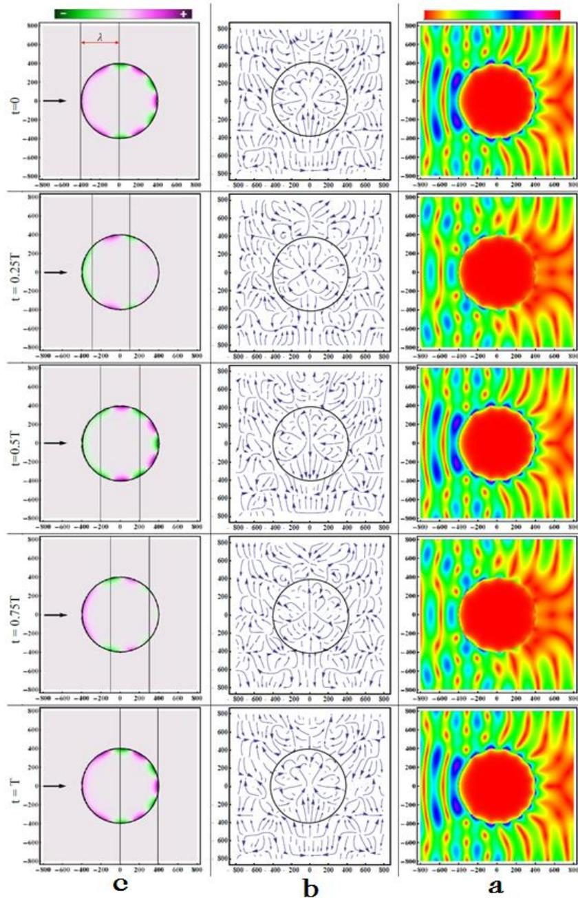
Fig. 5. Distribution of the field in and around a plasmonic nano-wires for different times. The electric field, (a) field lines, (b) and distribution of the charge density, (c). (axes are in nanometer).
