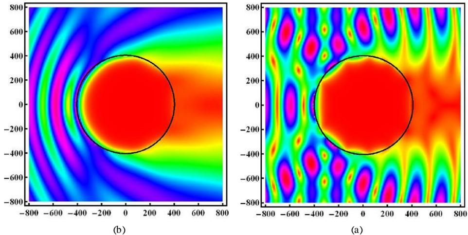
Fig. 3. TE polarized light scattering from a plasmonic nanowire, (a) the real part of the electric field, (b) the size distribution of the absolute value of the electric field (axes unit is nano-meter).
