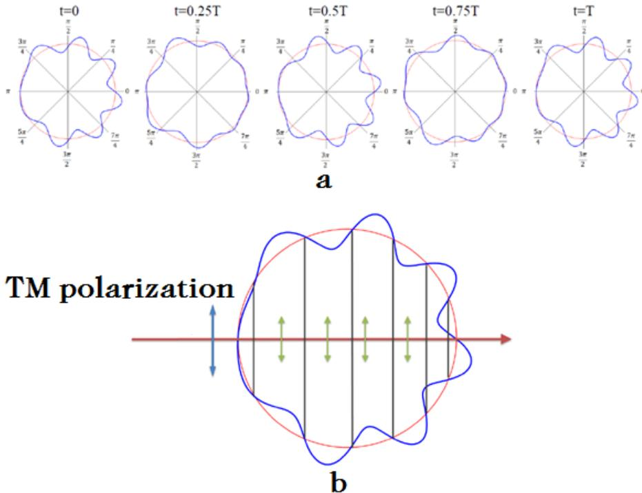
Fig. 6. Diagram of surface charge density on the boundary of nanowire. (a) For various times from 0 to  $T$  and (b) themmagnified diagram of time  $t = 0$ .
