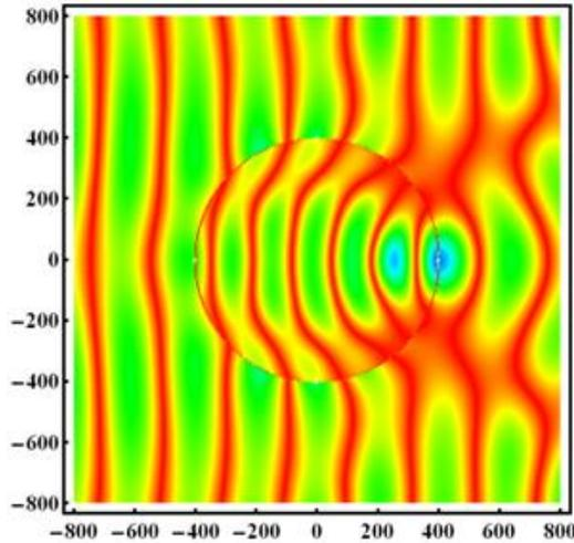
Fig. 2. Distribution of the electric field in and around a non-plasmonic nanowires under light with polarization TM (axes unit is nano-meters).
