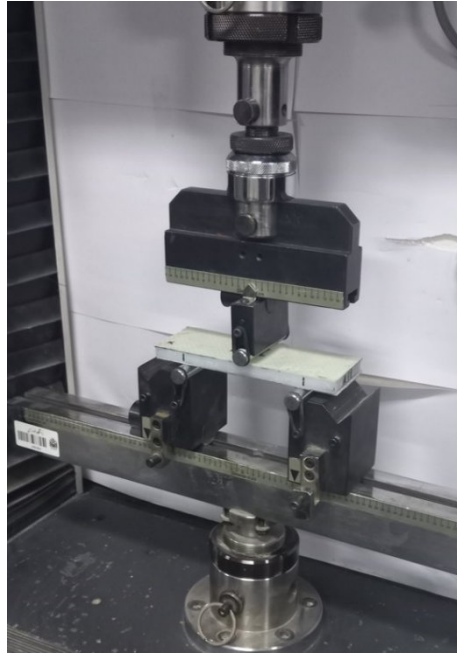
Fig. 3 Sandwich beam sample under a three-point bending test.
