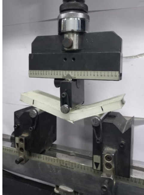
Fig. 7 Sandwich beam sample under a three-point bending test at the moment of failure.
