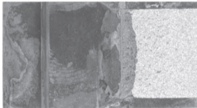
Fig. 4c Experimental observation of crack development pattern for the compact tension (CT) at load level 18kN. For more information, related to experimental data see [50].
