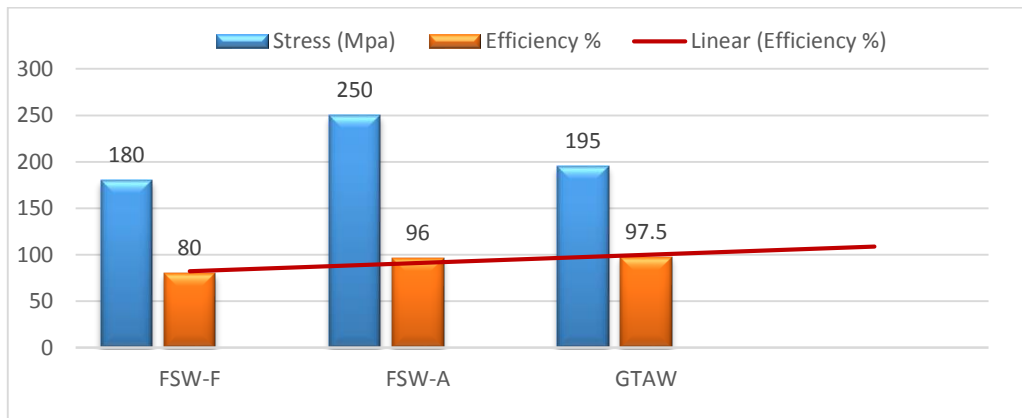
Figure 8. Graphical comparison of tensile test in FSW and TIG welding modes
