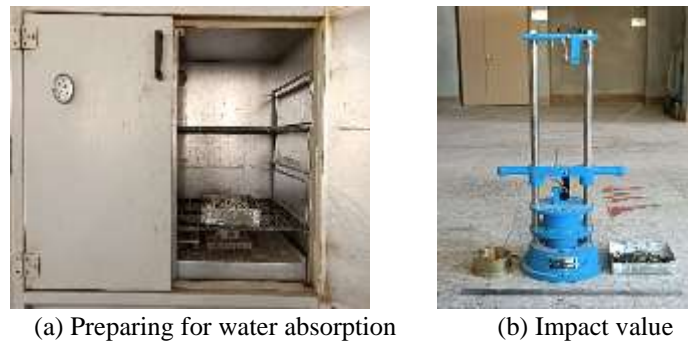
Fig. 4. Sample preparation and testing of samples
