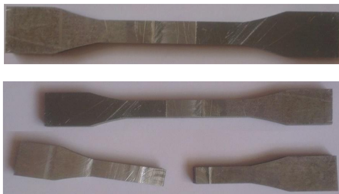
Figure 9. The sample used in the tensile test and the sample after the tensile test
