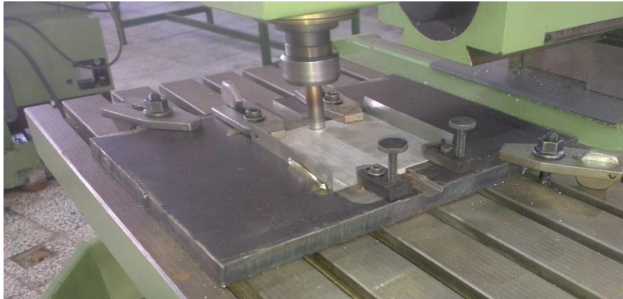
Figure 6. Implementation of the friction stir welding process
