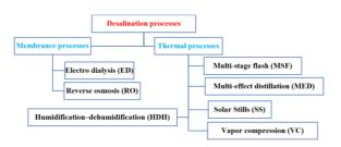
Fig. 1: Different methods of water desalination
