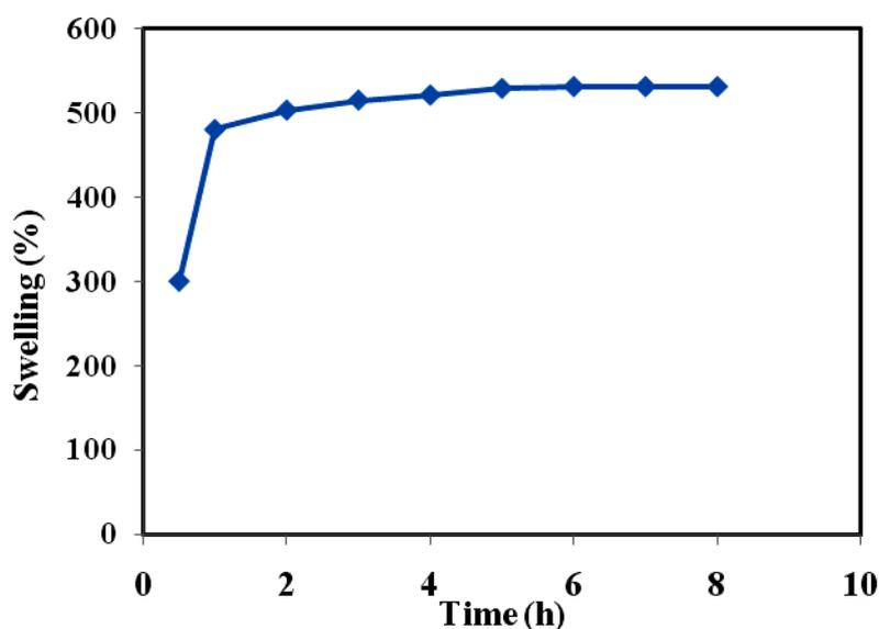
Figure 6. Degree of swelling versus immersion time (h) for nano-Fe<sub>3</sub>O<sub>4</sub>/PVA-SA hydrogel hydrogel at 25 °C.
