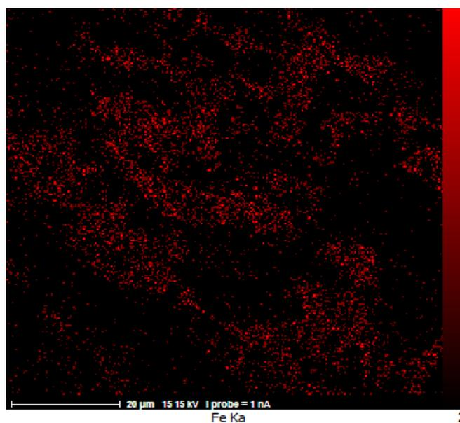
**Figure 3.** EDX distributions of nano- $\text{Fe}_3\text{O}_4$ /PVA-SA hydrogel.
