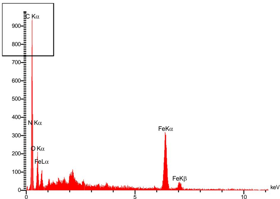
**Figure 4.** EDX spectra of magnetic PVA-SA hydrogel.
