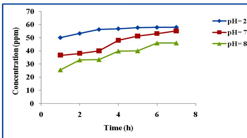
**Figure 8.** Concentration curve relative to time in different buffers at 37 °C.
