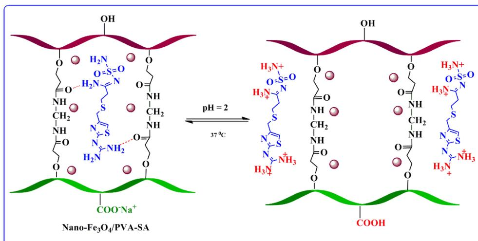
**Figure 9.** Proposed release mechanism of famotidine from nano-Fe<sub>3</sub>O<sub>4</sub>/PVA-SA hydrogel at pH=2.
