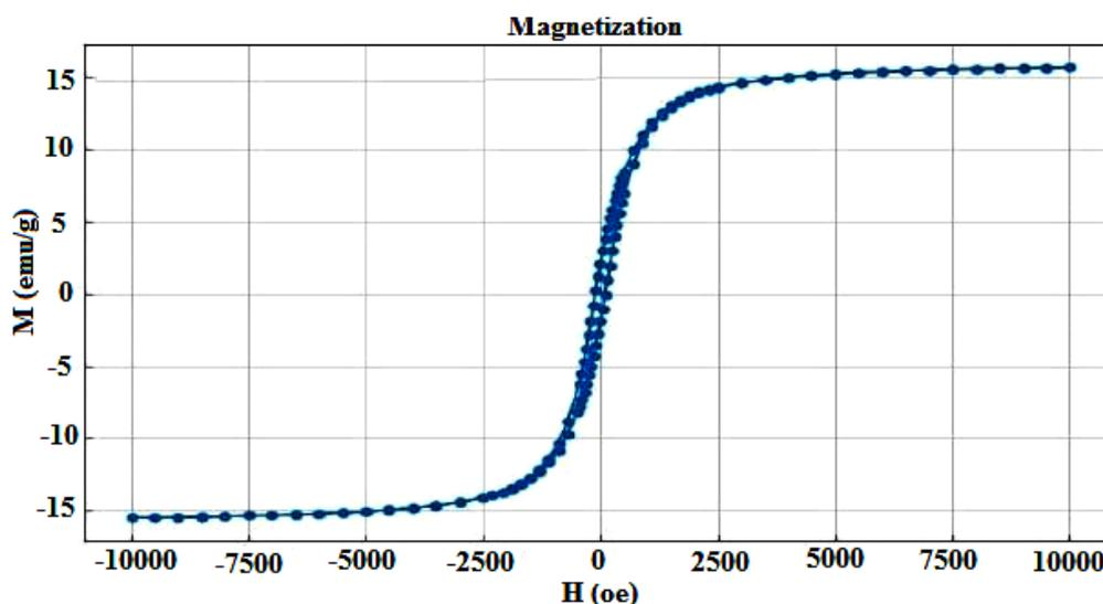
Figure 5. VSM magnetization curve of nano-Fe<sub>3</sub>O<sub>4</sub>/PVA-SA hydrogel.
