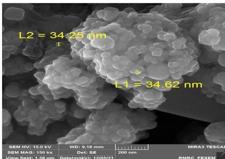
**Figure 2.** SEM image nano- $\text{Fe}_3\text{O}_4$ /PVA-SA hydrogel.
