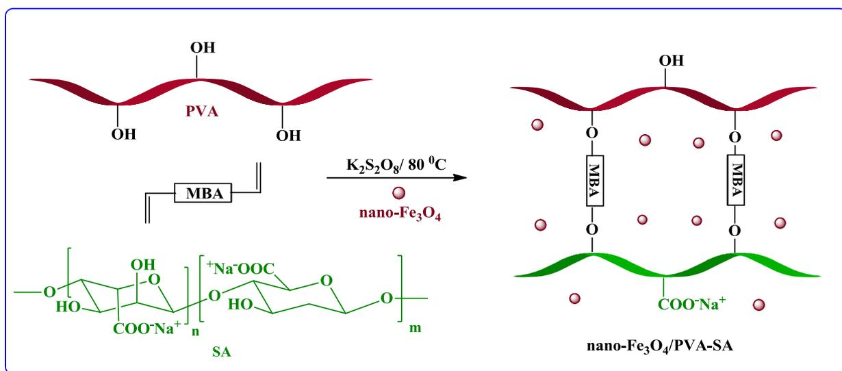
**Scheme 2.** The preparation of magnetic PVA-SA hydrogel.
