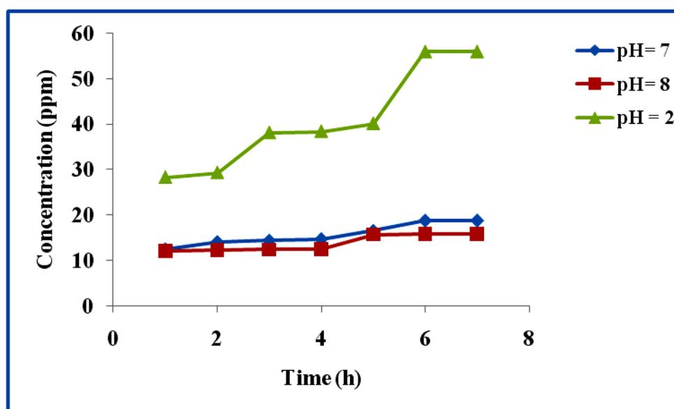
**Figure 7.** Concentration curve relative to time in different buffers at 25 °C.
