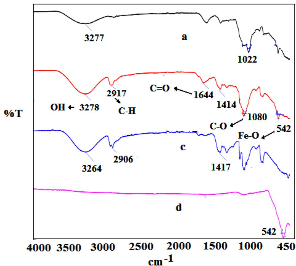
**Figure 1.** The FT-IR of, a- SA, b- nano-Fe<sub>3</sub>O<sub>4</sub>/PVA-SA, c- PVA, d- nano-Fe<sub>3</sub>O<sub>4</sub>.
