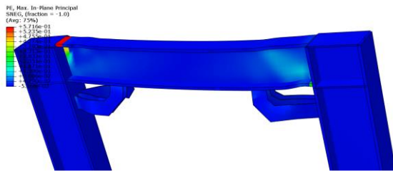
Figure 13-Plastic strain in the proposed connection
