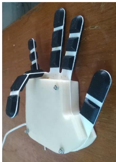
Figure 3. Flexi artificial hand made by 3D printing method
