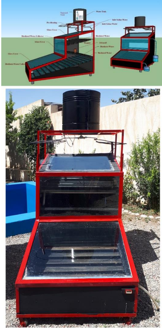
Fig. 1: Solar Water Desalination Device.
