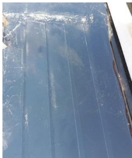
Fig. 2: The lower section of the stairs in the solar still
