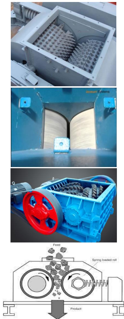
Fig. 1 The mechanism of roll stone crushers and different roller types
