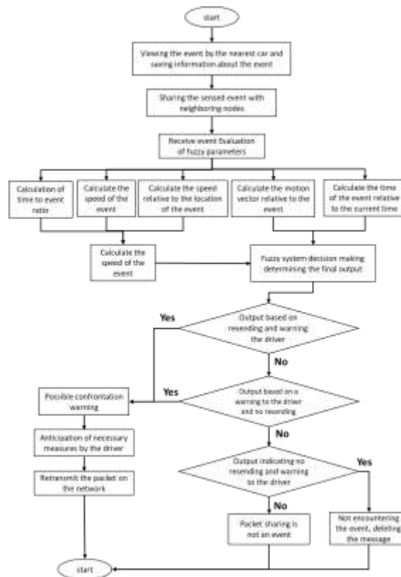
Fig. 3. The flowchart of the proposed method and its operational components.
