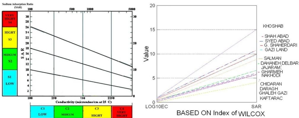
**Figure 2.** Classification of water quality based on the Wilcox Diagram EC was scaled on the horizontal axis and the SAR on the vertical axis of the diagram (Table 4)
