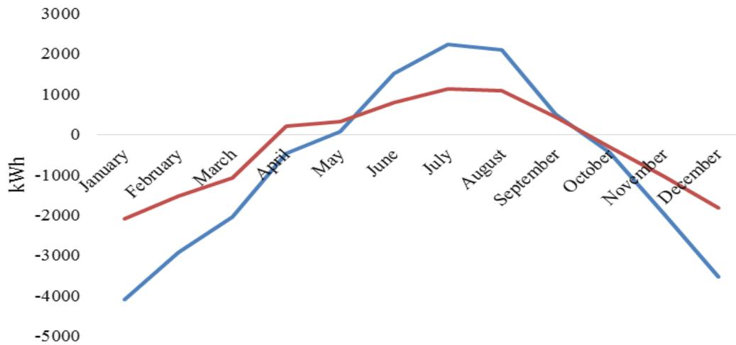
Figure 8. Heat transfer from the wall (Red line: optimal mode - Blue line: base mode)
