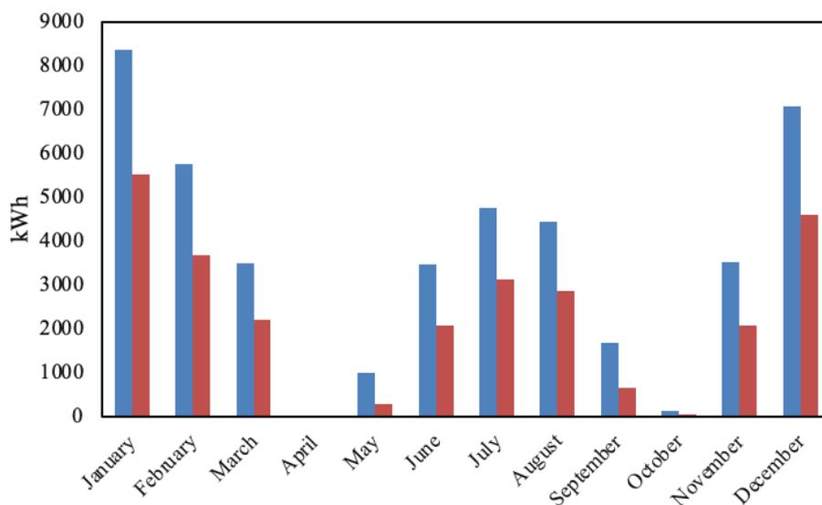
Figure 10. Comparison of total energy consumption of cooling and heating systems (Red line: optimal mode - Blue line: base mode)
