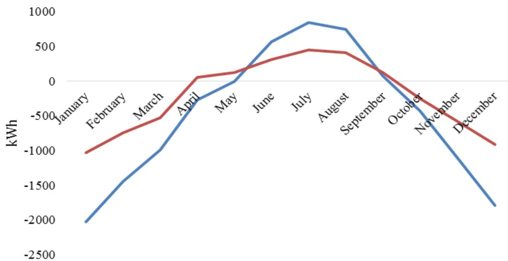
Figure 9. Heat transfer from the ceiling (Red line: optimal mode - Blue line: base mode)
