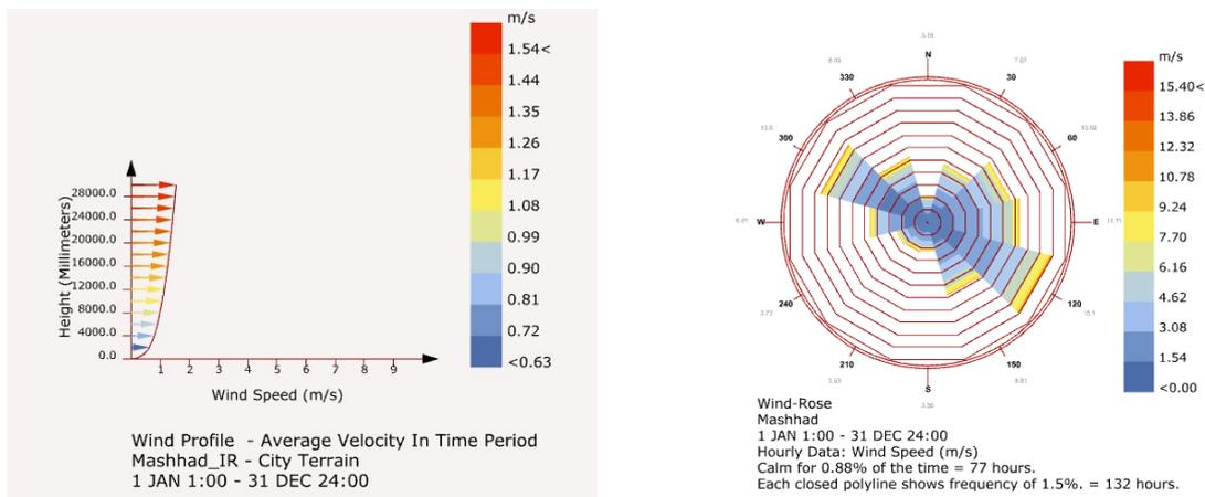
**Figure 7.** Mashhad Golbad diagram (right) and average wind speed diagram (left) (Source: research findings)
