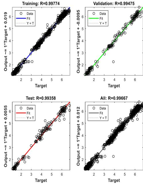
**Fig. 8** Regression of neural network error in ROP prediction for the 12 ¼-inch hole
