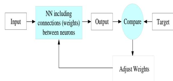
**Fig. 2** The training process of a neural network [26]
