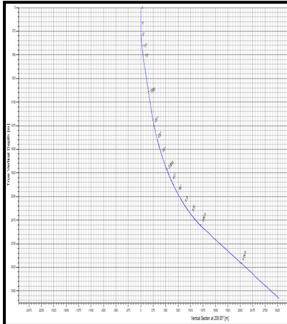
Fig. 3 The route designed for the studied well
