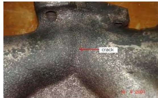
Fig. 15 The cracked exhaust manifold [33]
