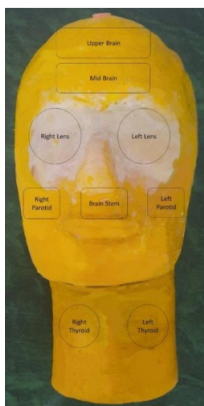
Figure 1. Head & neck phantom with the approximate position of considered organs.
