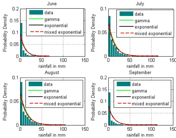
Figure 4. Histogram for June-September wet days and fitted exponential, gamma and mixed exponential probability density function for Dejen, Ethiopia.
