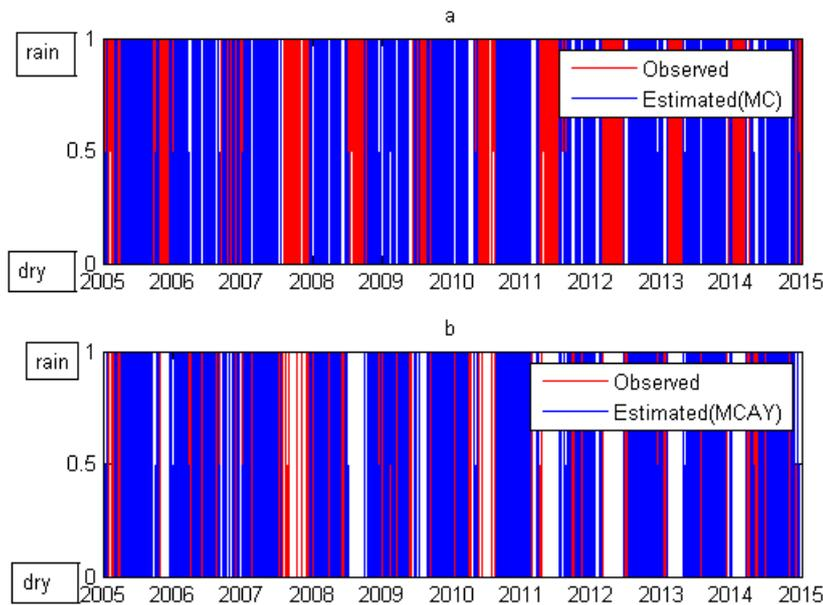
Figure 9. (a) Frequency of rainfall occurrence using MC (Markov chain with out analogue year component) (b) Frequency of rainfall occurrence using Markov chain with the analogue year component (MCAY) model.
