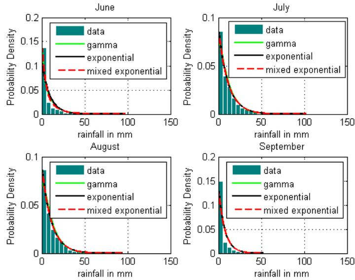
Figure 5. Comparison of the histogram of June-September wet days with Exponential, Gamma and mixed exponential probability density functions for Gonder, Ethiopia.
