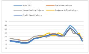
Fig. 4. Residential load profile at each scenario in a day
