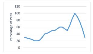
Fig. 2. Load profile of benchmark LV feeder in one day
