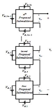
Fig. 2. Cascade proposed structure
