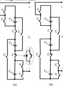
Fig. 1. a) first and b) second proposed Submultilevel inverters
