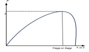
Fig. 1. Characteristic of PV panel power curve.
