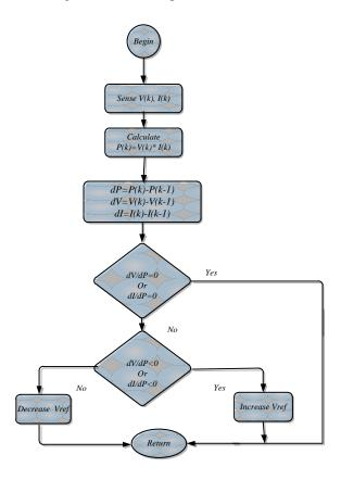
Fig. 3. Block diagram of incremental conductance method
