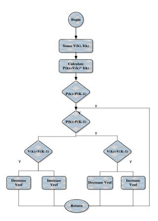
Fig. 2. Block diagram of P&O method
