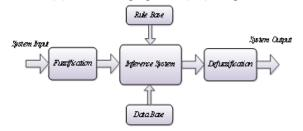
Fig. 4. Block diagram of fuzzy logic controller.
