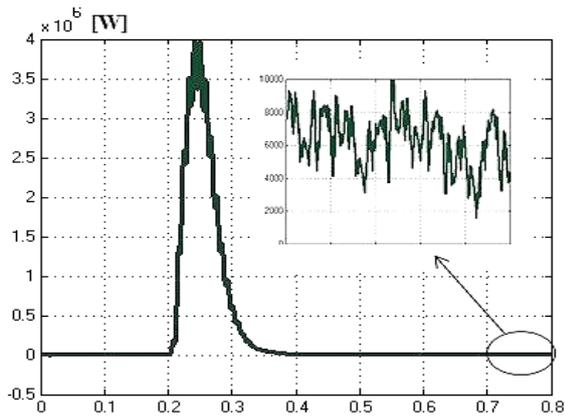
Fig. 6. Instantaneous active power of the Trasformerless SSSC
