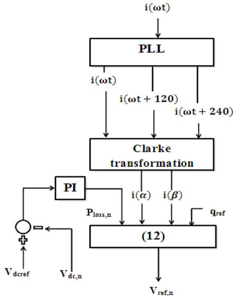
Fig. 4. The block diagram of the Control algorithm
