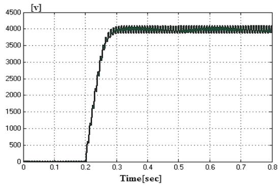
Fig. 11. Dc link voltage of each bridge of the inverter in phase a
