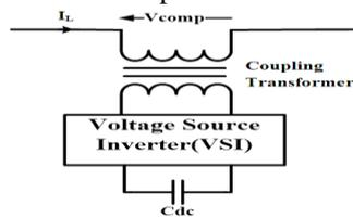
Fig. 1. Structure of SSSC
