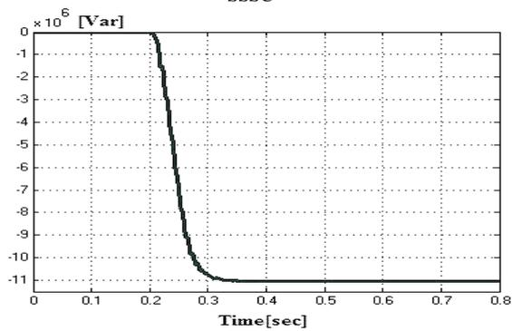
Fig. 7. Instantaneous reactive power of the Trasformerless SSSC
