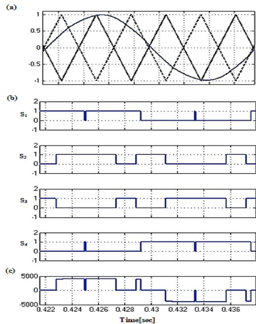
Fig. 5. P-S PWM technique to create switching signals for each bridge of CHB inverter: (a) carrier signals, (b) switching pattern, (c) equivalent modulated Signal
