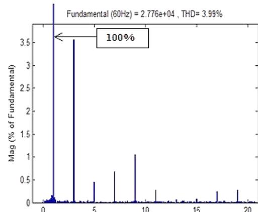
Fig. 10. FFT analysis of the waveform of the phase a voltage
