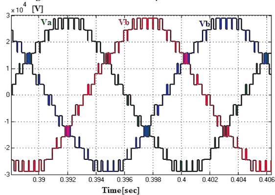
Fig. 9. Three-phase output voltage waveforms of the Trasformerless SSSC
