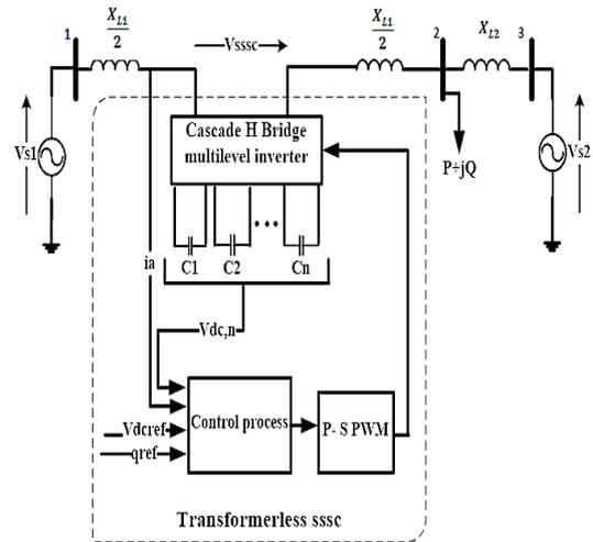
Fig. 2. Single line diagram of the proposed system
