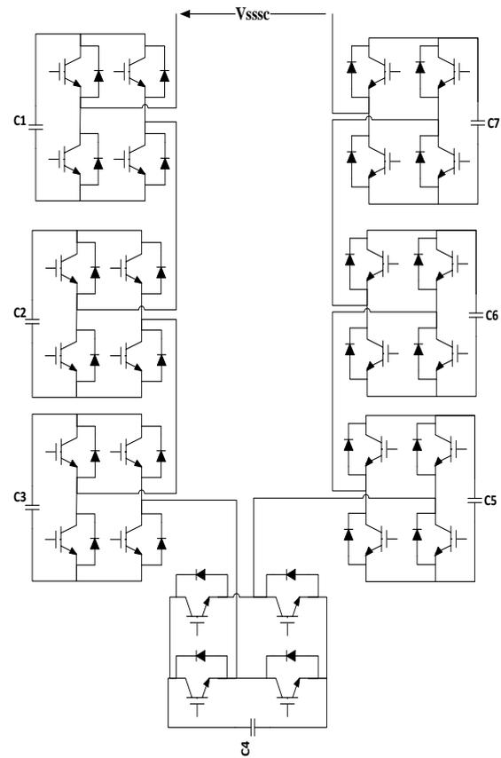
Fig. 3. Configuration of the multilevel inverter
