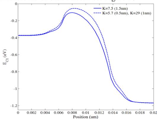
Fig. 15. The conduction band energy in the on state ( $V_{GS} = V_{DS} = 0.8V$ ).
