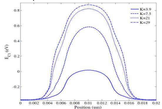
Fig. 10. The first band sub-band energy for the proposed device in thermal equilibrium and different  $K$  values.
