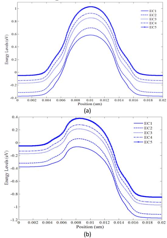
Fig. 7. Energy levels for the proposed device with  $K = 7.5$  in (a) thermal equilibrium condition ( $V_{DS} = V_{GS} = 0V$ ) and (b) for on state condition ( $V_{DS} = V_{GS} = 0.8V$ ).
