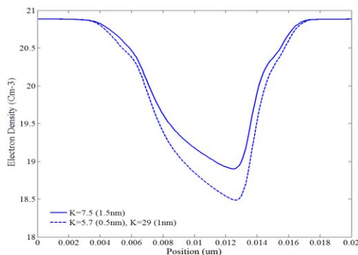
Fig. 16. Electron density along the channel for simulated structure
