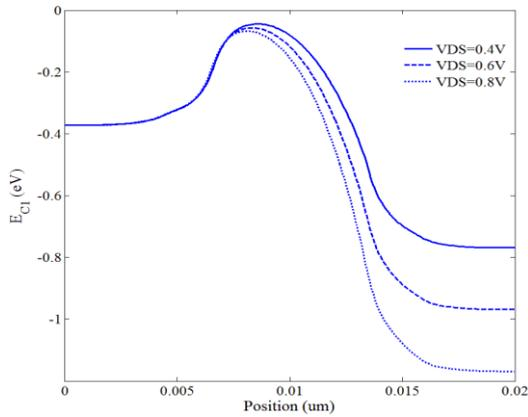
Fig. 5. The first sub-band energy along the channel for different values of V<sub>DS</sub>.
