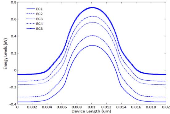
Fig. 2. The conduction sub-bands energy of the proposed device at the thermal equilibrium
