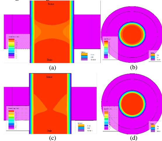
Fig. 4. Electron density (a) and direction of electron motion (b) in the direction perpendicular to the motion of the electron at zero ( $V_{GS} = V_{DS} = 0V$ ). Electron density (c) and direction of electron motion (d) in the direction perpendicular to the motion of the electron in the on-state ( $V_{GS} = V_{DS} = 0.8V$ ).
