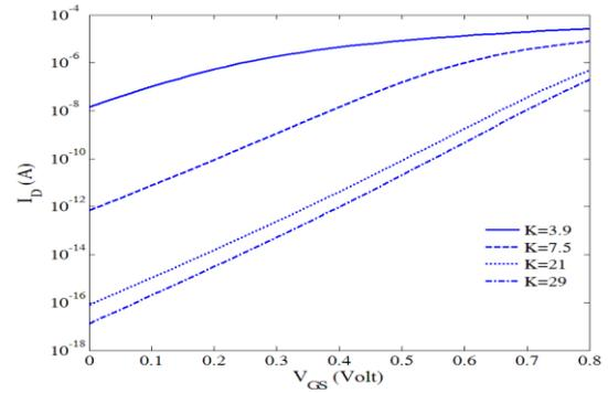
Fig. 9. ID-VGS characteristic for the proposed structure for different values of  $K$
