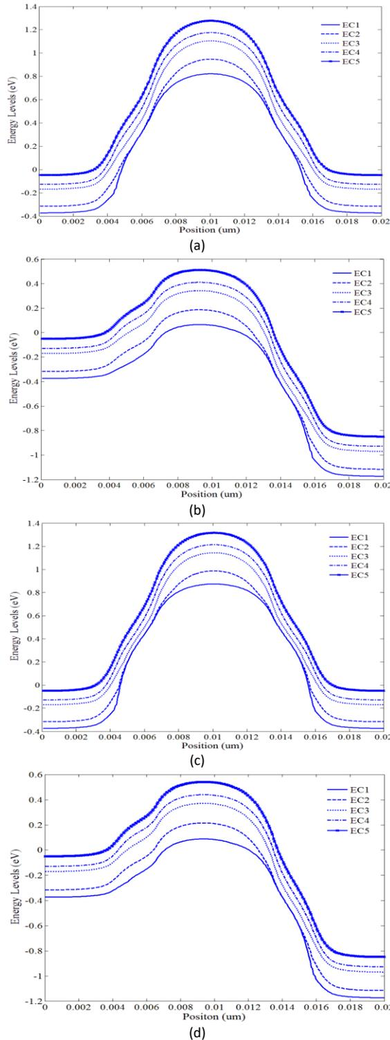
Fig. 8. Energy levels for  $K = 21$  in (a) thermal equilibrium and (b) in the on state and for  $k = 29$  in (c) thermal equilibrium and (d) in the on state.
