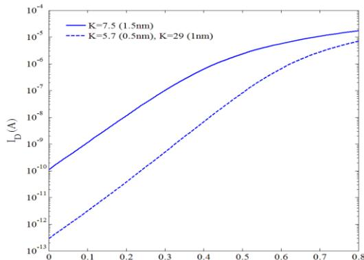
Fig. 14. Input characteristics of the GAA-JL-FET-with-oxide buffer layer
