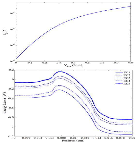
Fig. 3. The ID-VGS curve and The sub bands energy level along the device at the on state
