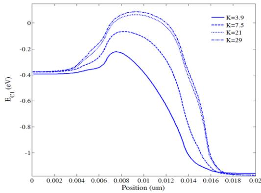
Fig. 11. The first sub-band of the conduction band for the proposed device in the on state for different values of K.
