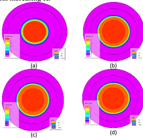
Fig. 12. Electron density in the on state at the cross section perpendicular to the current flow in the center of the gate for the values of (a) K = 3.9, (b) K = 7.5, (c) K = 21 and (d) K = 29.
