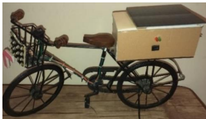
Fig. 7. Making a maquette of a smart solar bike with a sterile box mounted on the bike
