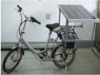
Fig. 5. Prototype bicycle with solar energy 12V / 50W
