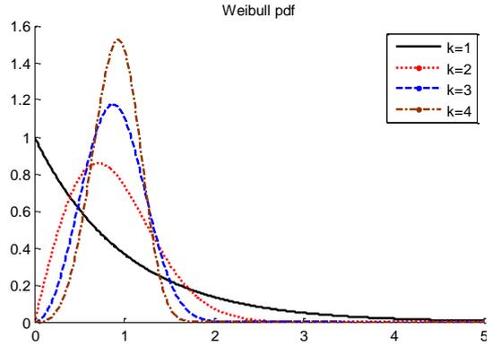
Fig. 2. Weibull pdf with different shape index (c=1)
