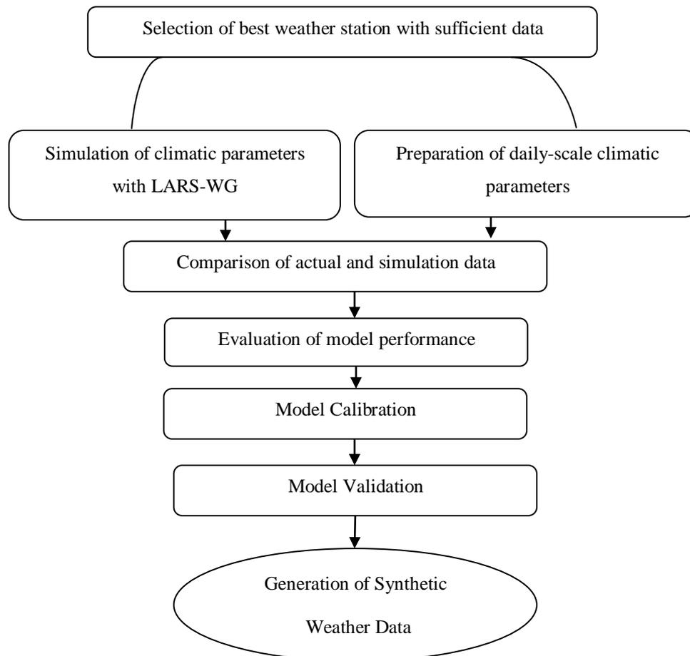
Fig. 2. Research method diagram
