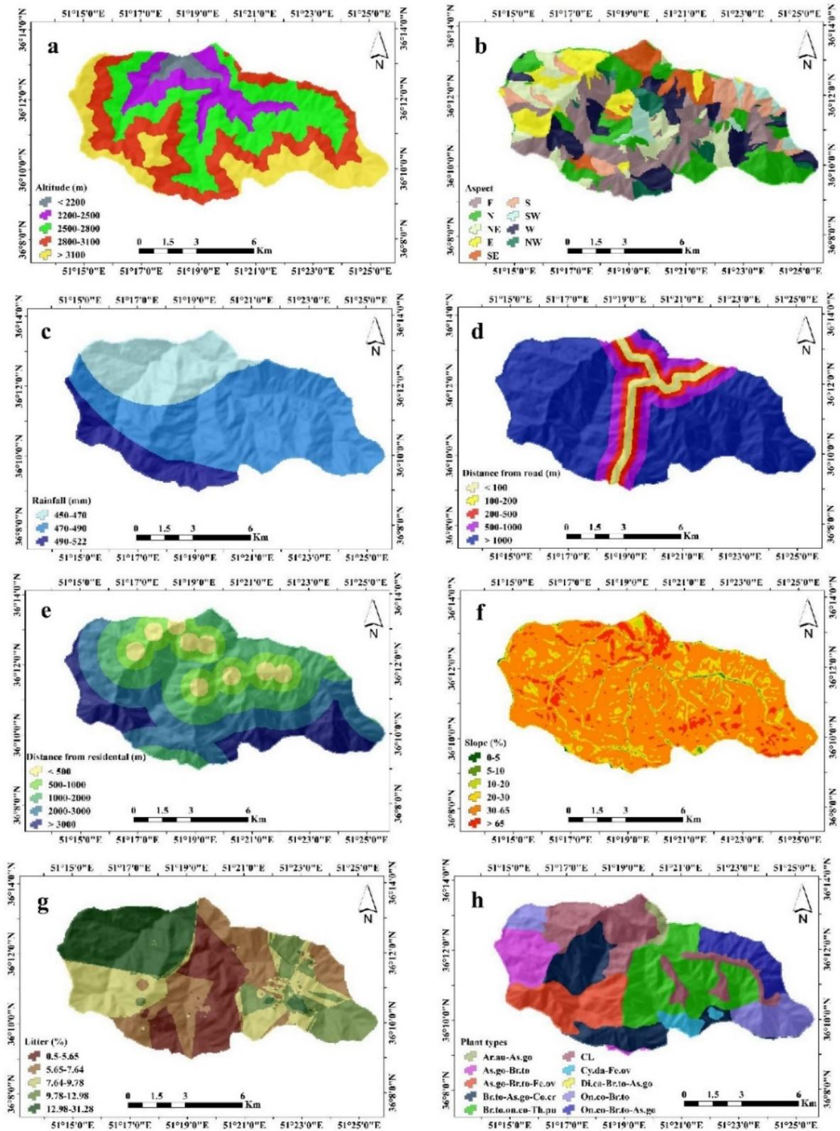
**Figure 2.** Influential variables used in the rangeland fire (a) Altitude (b) Aspect (c) Rainfall (d) Distance from road (e) Distance from residential (f) Slope (g) Litter (h) Plant type.
