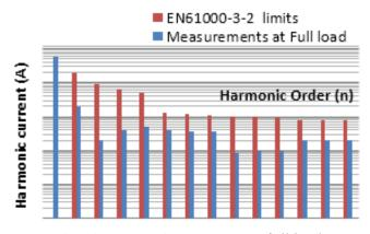
Fig. 10. Harmonics spectrum at full load.
