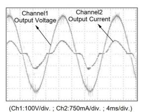
Fig. 6. Output voltage and current for a nonlinear load (135 W).
