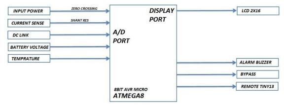
Fig. 2. Control, display and alarm unit.
