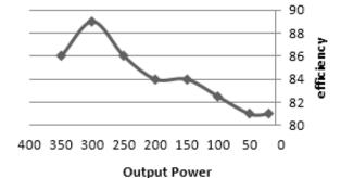
Fig. 9. Efficiency against output power variation of UPS.
