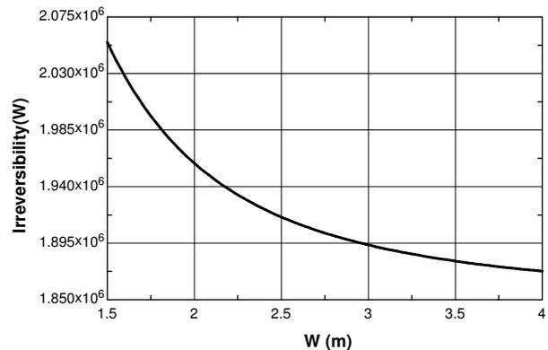
Fig. 7. Sensitivity analysis for width of the steam generator
