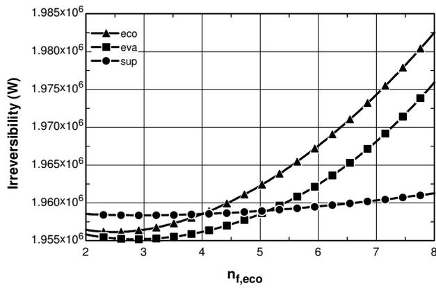
Fig. 10. Sensitivity analysis for the number of fins per inch in the economiz
