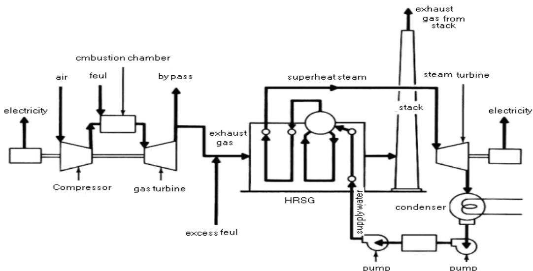
Fig. 1. Schematic of a combined cycle power plant
