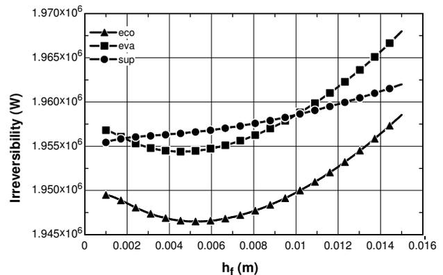
**Fig. 9. Sensitivity analysis for height of fins of the economizer**
