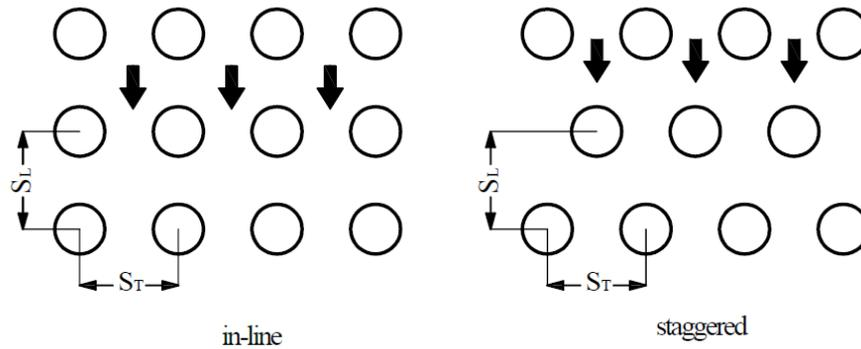
Fig. 3. Arrangement of tubes in heat recovery steam generators
