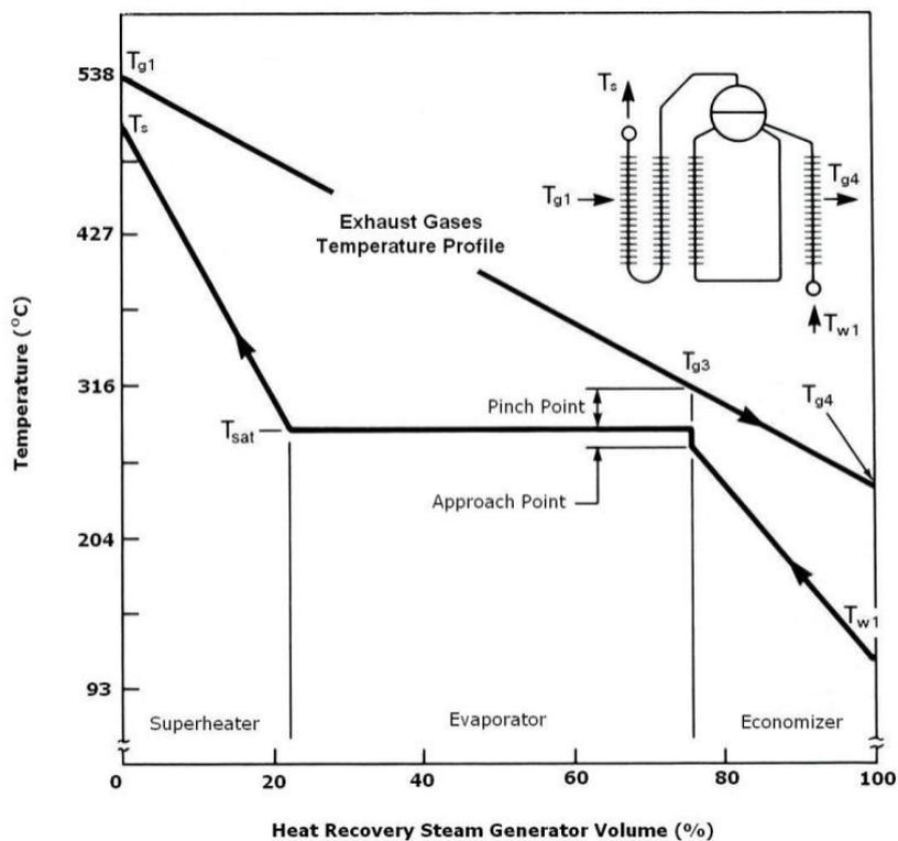
Fig. 2. Temperature profile in a heat recovery steam generator
