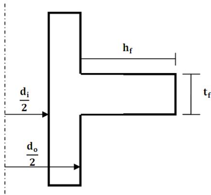
Fig. 4. Schematic of fin geometry
