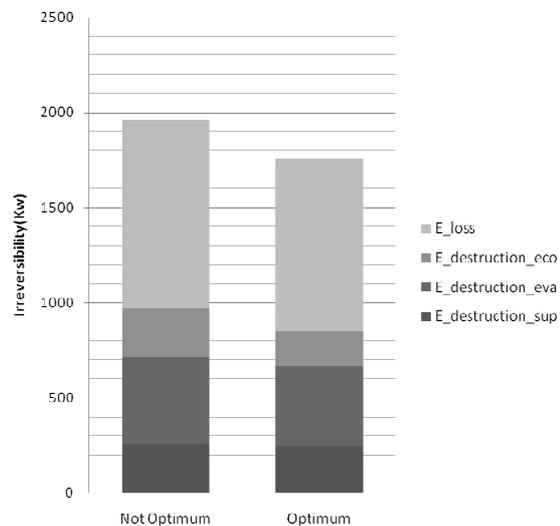
Fig. 12. Irreversibility in each of the parts of the generator, before (left) and after (right) the optimization
