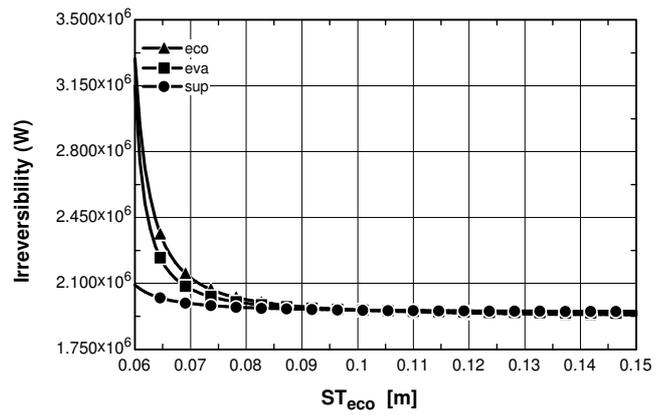
Fig. 11. Sensitivity analysis for transverse pitch of the fins in the economizer
