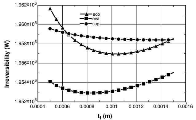
**Fig. 8. Sensitivity analysis for thickness of fins of the economizer**
