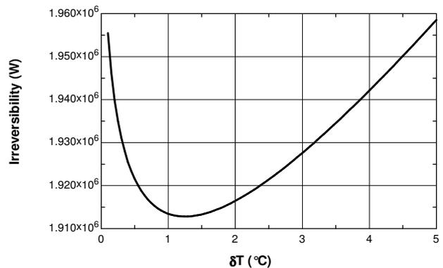
Fig. 6. Sensitivity analysis for pinch temperature difference
