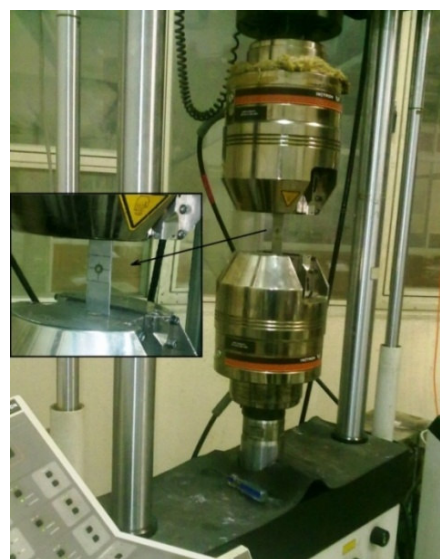
Fig. 2. Specimen position between grippers.
