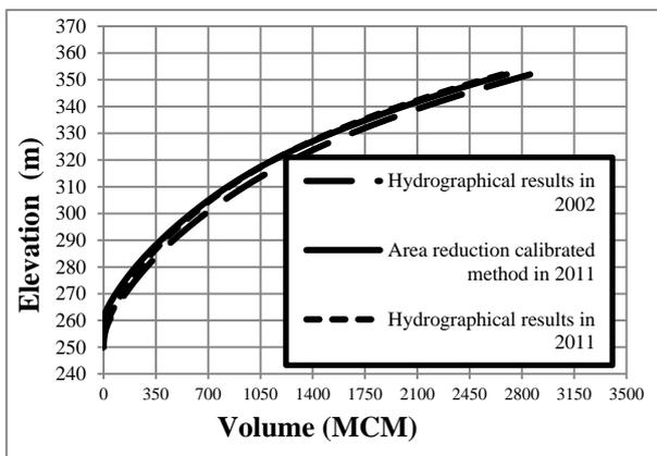
Fig.9. Running area-reduction calibrated through MATLAB & GA Combined Model in 2011
