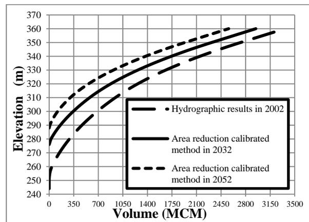
Fig. 10. Running the area-reduction calibrated MATLAB & GA Combined Model for 2032 and 2052
