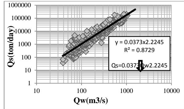
Fig.2. Dez Dam sediment rating curve (suspended load)
