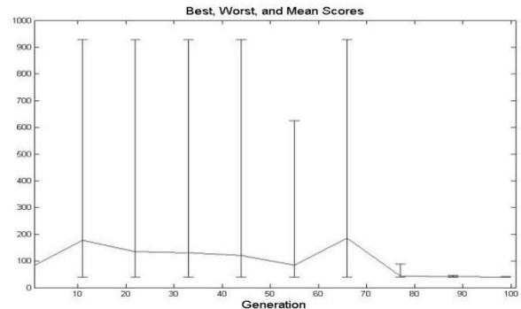
Fig.7. The best, worst and mean scores diagram due to the generation in calibration of the three parameters by GA
