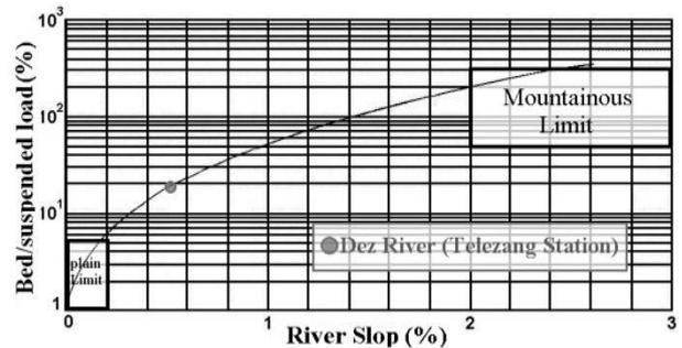
Fig.3. Karashev Experimental Curve to estimate bed to suspended load ratio
