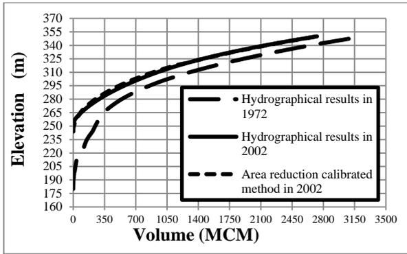
Fig.8. Running area-reduction calibration through MATLAB & GA Combined Model in 2002
