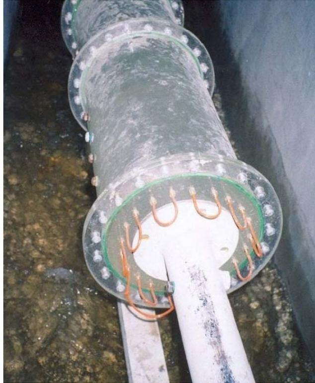
Fig. 2. Picture of sudden pipe expansion
