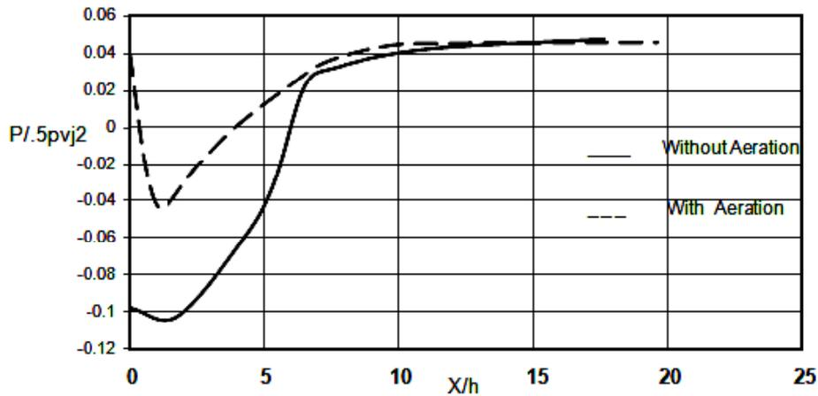
Fig. 7. Mean static pressure distribution on the centre line of the jet
