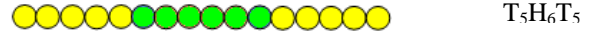
Fig. 1. Gemini surfactant. Yellow circles represent hydrophobic tail segments and green circles represent hydrophilic segments (head or spacer).
