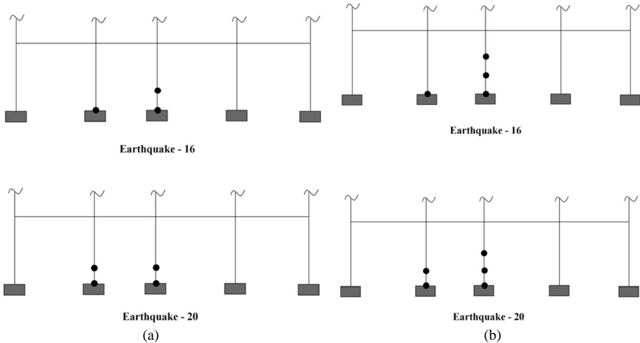
Figure 9. Plastic hinge formation in the boundary frames for the upgraded: a) 7-story; and b) 5-story frames
