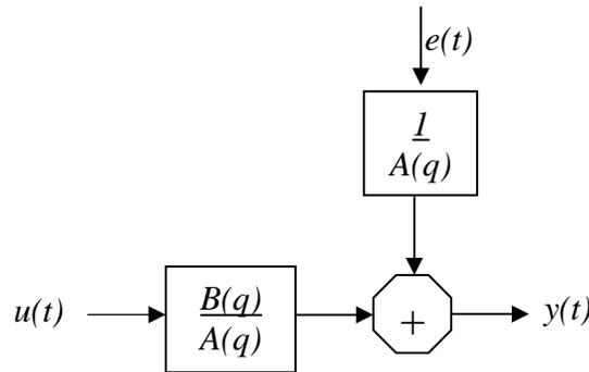
Figure 2. The ARX model structure
