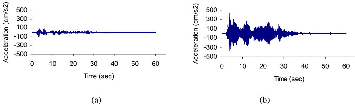
Figure 6. El Centro 1940 NS record with a velocity target of story stiffness: a) Input wave at base level; b) Measured response at third story level
