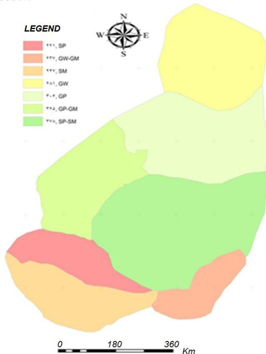
Figure 6. Map of allowed bearing capacity with 1 m dimensions at a 1 m depth
