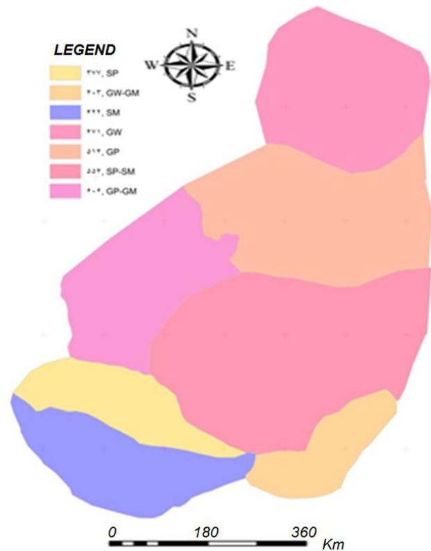
Figure 7. Map of allowed bearing capacity with 2 m dimensions at a 1.5 m depth
