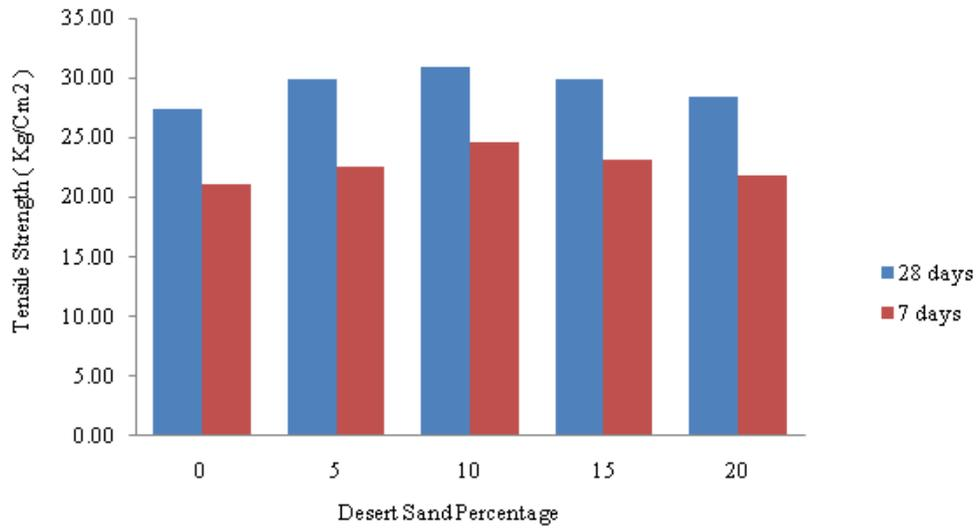
Figure 7. Tensile Strength for C20
