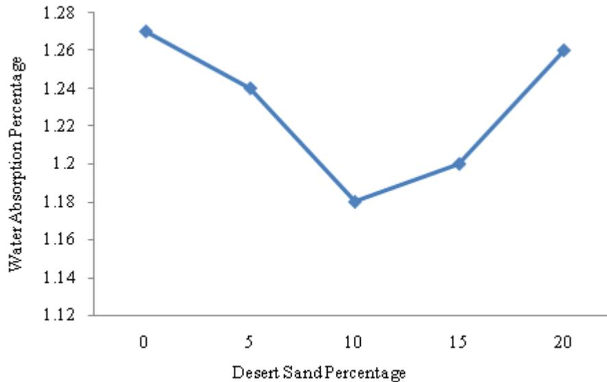
Figure 10. Water Absorption of C25 Specimens
