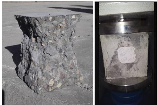
**Figure 3.** Breakage condition of compressed specimens
