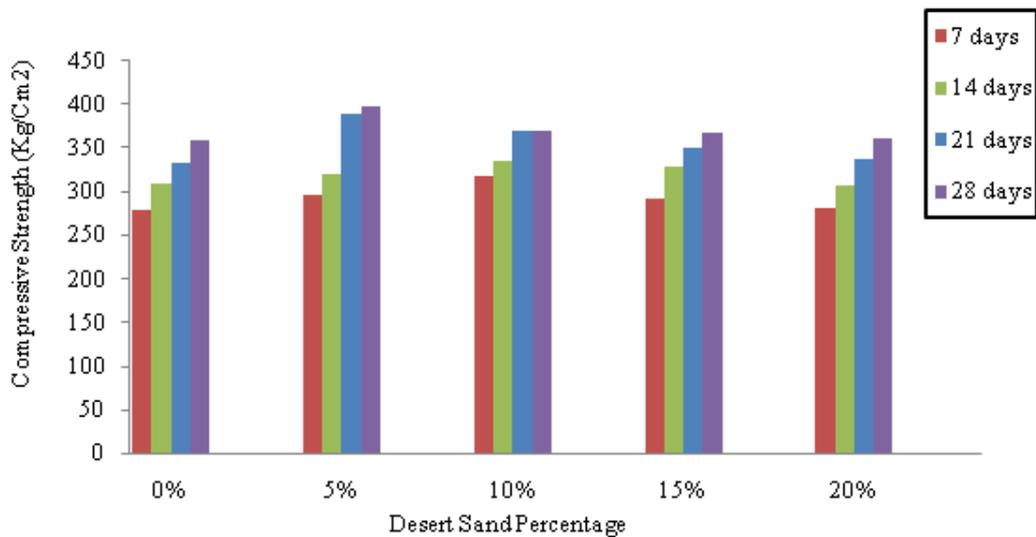
Figure 6. Compressive Strength of C30 Concrete
