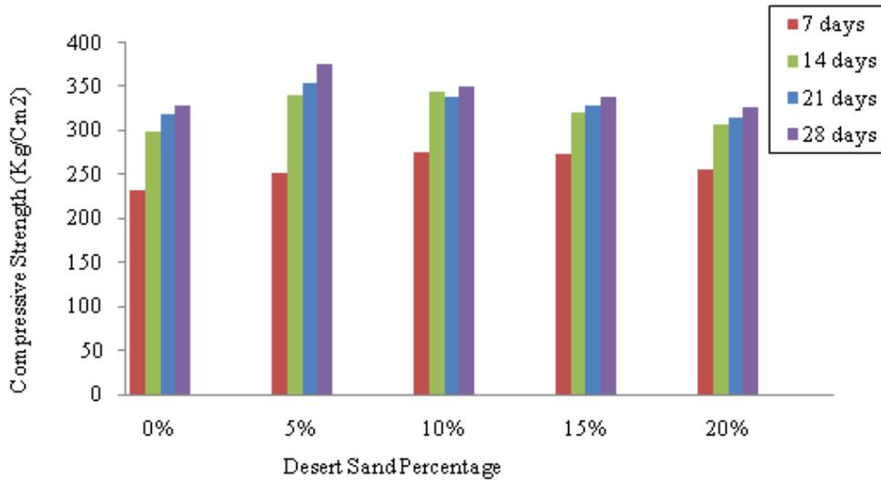
Figure 5. Compressive Strength of C25 Concrete
