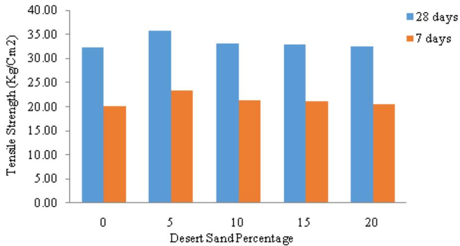
Figure 9. Tensile Strength for C30
