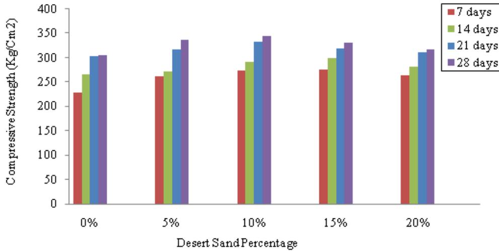
Figure 4. Compressive Strength of C20 Concrete
