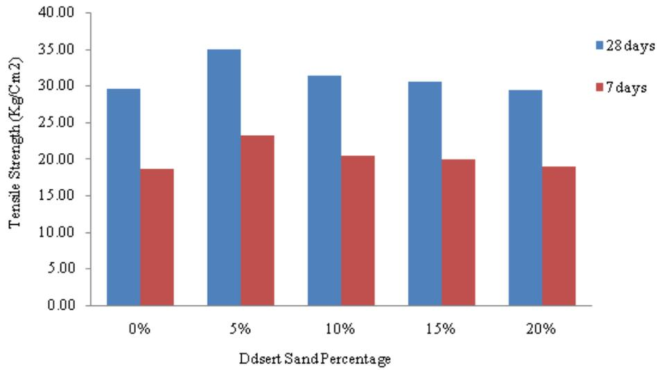
Figure 8. Tensile Strength for C25
