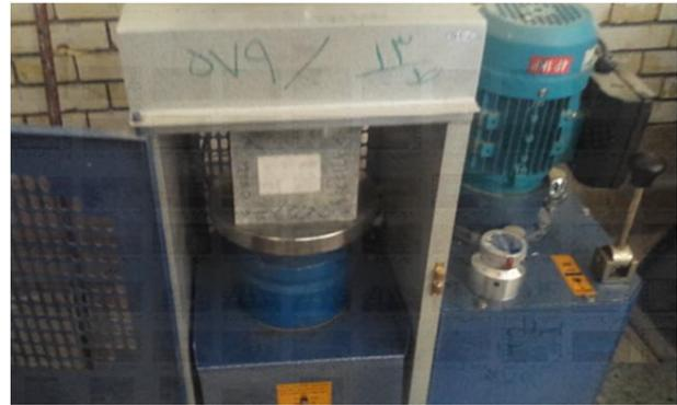
**Figure 1.** A view of used compressive strength test (UCS)
