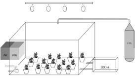
Fig. V. Set-up of the labeling chamber for isotopic labeling of whole plants (Sanchez et al, 2000)
