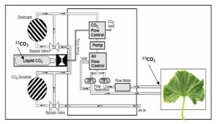
Fig. III. LI-6400 open system of photosynthetic gas exchange (IRGA); the incoming air stream can be conditioned for  $CO_2$  concentration, humidity, and temperature. There are chemical tubes for scrubbing  $CO_2$  and  $H_2O$ . The air was diverted through these tubes and  ${}^{12}CO_2$  from the incoming air was removed, and  ${}^{13}CO_2$  source injected to system.
