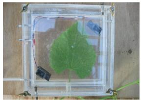
Fig.II. Single leaf labeling chamber with approximately 350 cm2 size (Barzegar, 2011).
