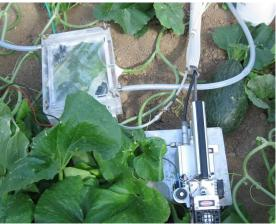
Fig. I. Labeling chamber coupled to the Licor-6400 gas exchange system (Barzegar, 2011).
