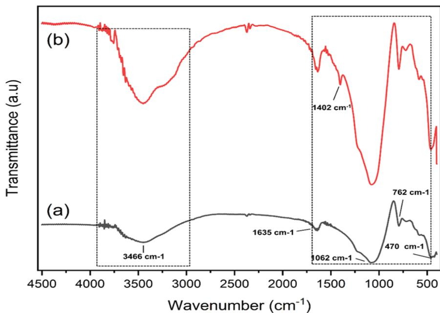
Fig. 5 FTIR spectra of (a) zeolite-Zr and (b) zeolite-Zr(H<sub>2</sub>PO<sub>4</sub>)<sub>4</sub>
