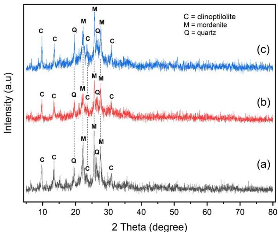
**Fig. 2** XRD spectra of (a) NZ (b) NZ-Zr (c) NZ-Zr(H<sub>2</sub>PO<sub>4</sub>)<sub>4</sub>
