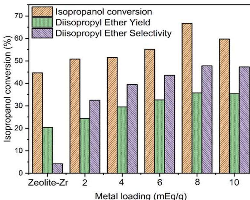
**Fig. 7** The isopropanol conversion, DIPE yield, and selectivity catalyzed by zeolite-Zr and zeolite-Zr(H<sub>2</sub>PO<sub>4</sub>)<sub>4</sub> at various metal loading
