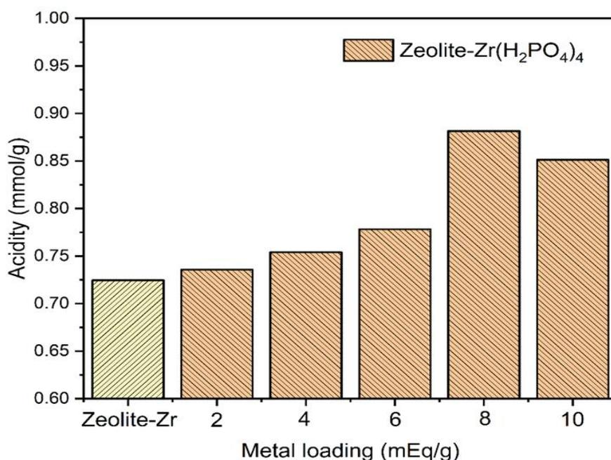
**Fig. 6** Acidity of zeolite-Zr and zeolite-Zr(H<sub>2</sub>PO<sub>4</sub>)<sub>4</sub> with various metal loading
