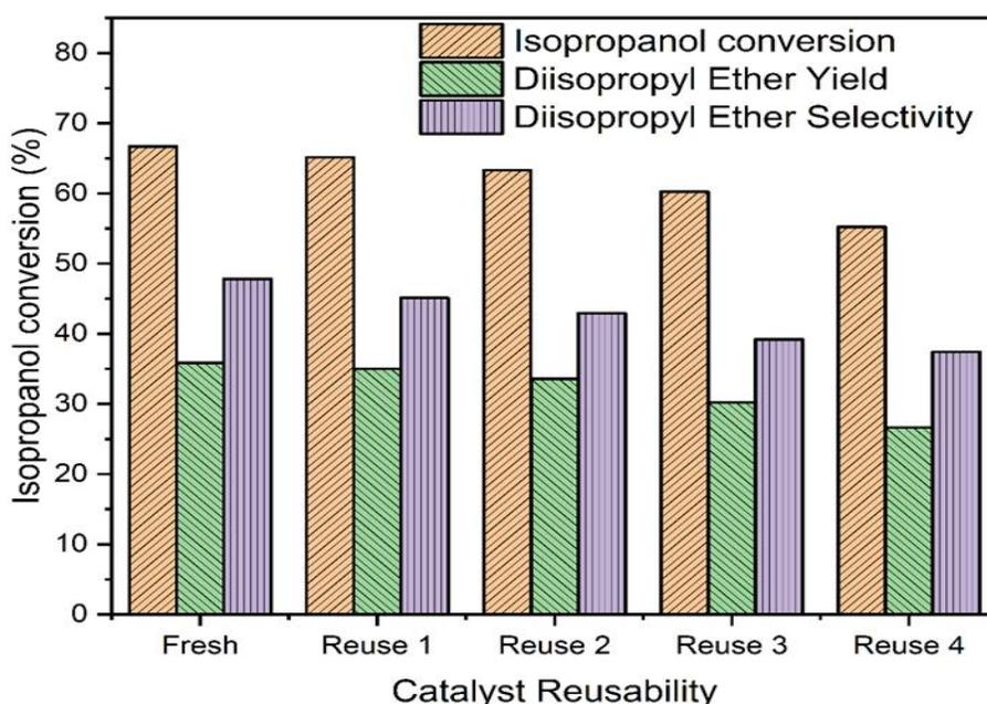
**Fig. 8** Reusability of zeolite-Zr(H<sub>2</sub>PO<sub>4</sub>)<sub>4</sub> catalyst
