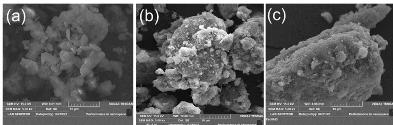
**Fig. 3** SEM images of (a) NZ (b) NZ-Zr (c) NZ-Zr(H<sub>2</sub>PO<sub>4</sub>)<sub>4</sub>
