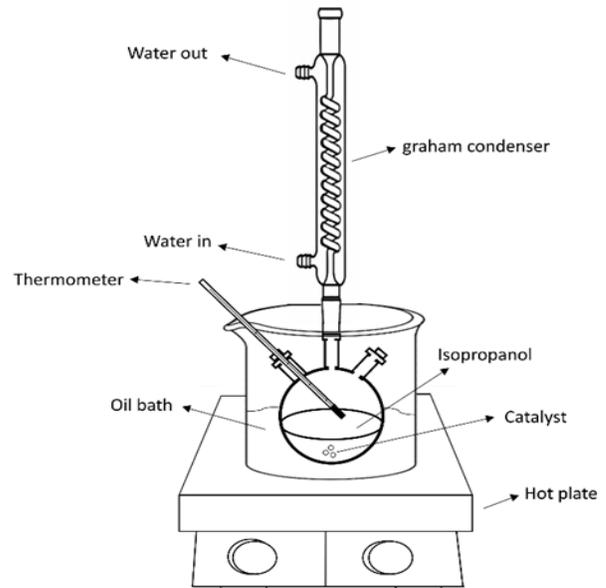
**Fig. 1.** Schematic diagram of dehydration reaction
