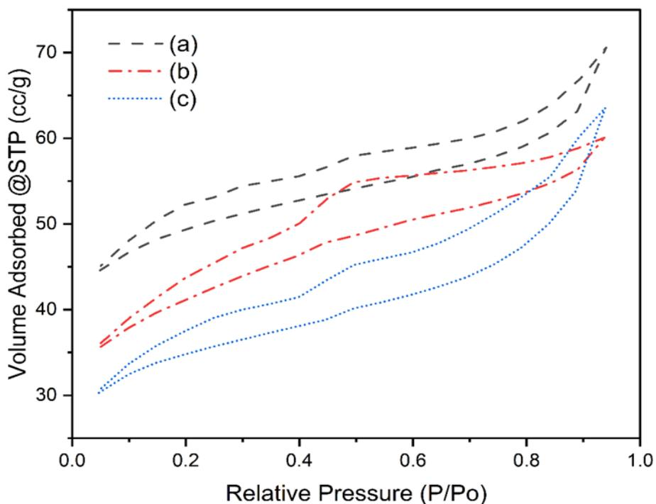
Fig. 4 N<sub>2</sub> physisorption of (a) NZ(b) NZ-Zr and (c) NZ-Zr(H<sub>2</sub>PO<sub>4</sub>)<sub>4</sub>
